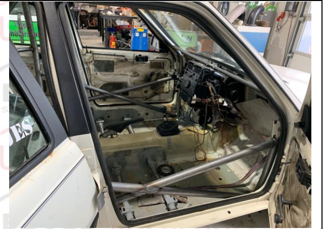
PHOTO 11 ANTI-INTRUSION DOORBAR – CO-DRIVER
