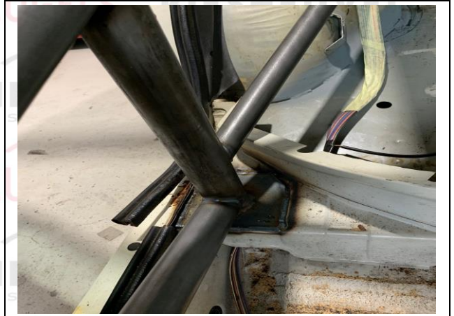
PHOTO 4 MAIN ROLLBAR TO FLOOR ATTACHMENT
