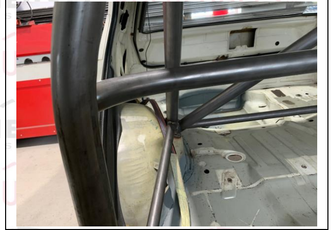
PHOTO 13 SHOULDER HARNESS ATTACHMENT - CO DRIVER
