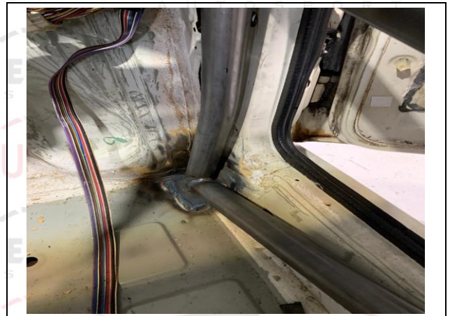
PHOTO 6 FRONT ROLLBAR TO FLOOR ATTACHMENT
