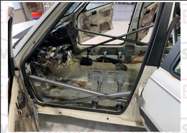
PHOTO 10 ANTI-INTRUSION DOORBAR - DRIVER
