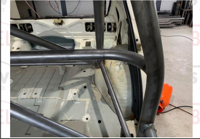
PHOTO 12 SHOULDER HARNESS ATTACHMENT - DRIVER
